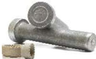
The UNBRAKO ARC Welding Stud also known as Shear Connector is used in the construction of tall buildings, bridges and steel structures. Drawn-arc process is used for stud welding. It improves the strength of the structure.
