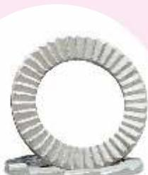
The Durlok® washer when used in combination with standard hex helps achieve self-locking properties. It is an anti-vibration solution that not only prevents bolted joint failure, but also enables the bolted joint to retain its pre-load, thus reducing maintenance requirements. The test regime highlighted this feature (fig 1).
