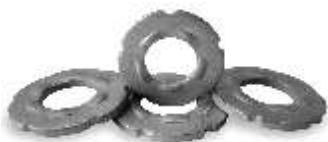
UNBRAKO Direct Tension Indicators, also known as Auto Torque Indicators, are single-use mechanical load cells designed to indicate the magnitude of preload in the assembly. It shows if the bolt is properly tensioned, very useful while tensioning High Strength Structural Bolts.
