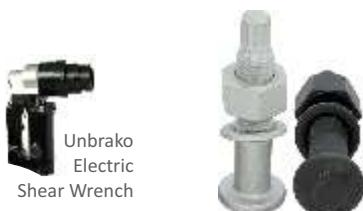
UNBRAKO Auto Torque Check Bolt also known as Tension Control Bolt is an easy to install Heavy Duty Bolt used in Steel Frame Construction. It has its own built-in torque control device. The outer socket of wrench rotates the nut until the torque control groove in the spline shears off on achieving proper bolt tension.
